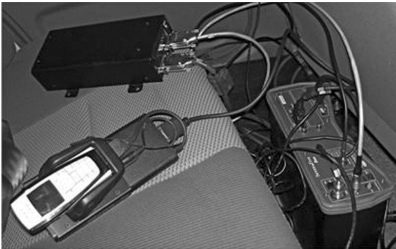
Figure 20.12 Comarco radio network measurement equipment connected to basic GSM test phone. The respective scripts are used for the testing, including data and voice call initiation, maintaining and terminating according to wanted time intervals.
