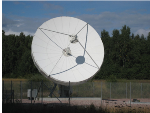
Figure 24.6 A fence around the antenna of a satellite ground station is a good idea also from the RF radiation safety perspective. Photo by Jouko Rautio.
