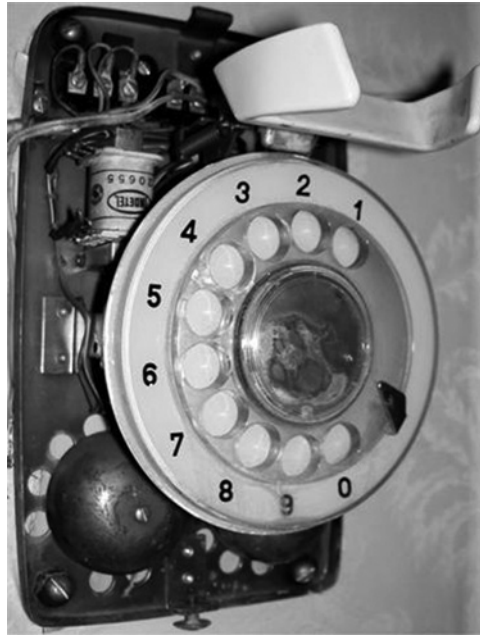
Figure 6.7 An example of wall-mounted analog telephone equipment, the inner parts exposed.
