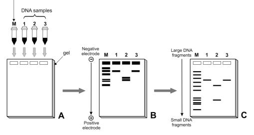
Figure 2.15 Gel electrophoresis. **A** DNA mixed with dye is loaded into wells in a gel; **B** an electric field is applied and the DNA fragments begin to move through the gel at different speeds according to their size; **C** different DNA fragments are separated by size, with the smallest fragments having moved the furthest along the gel
