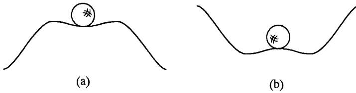
Figure 118 Limitations of a local stability criterion
