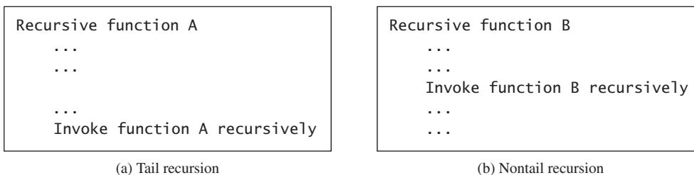
**FIGURE 15.13** A tail-recursive function has no pending operations after a recursive call.
