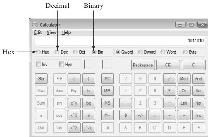
**FIGURE C.1** You can perform number conversions using the Windows Calculator.
