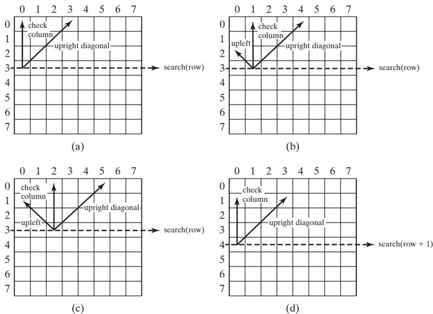
**FIGURE 15.12** Invoking `search(row)` fills in a queen in a column in the row.
