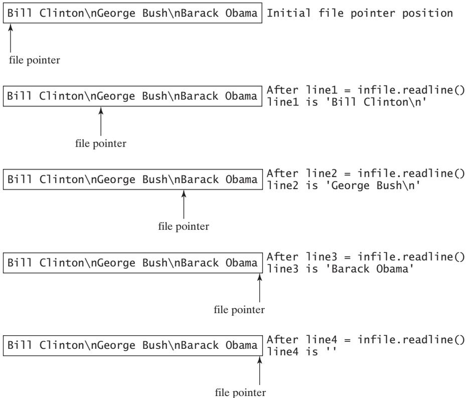
**FIGURE 13.5** The `readline()` method reads a line.
