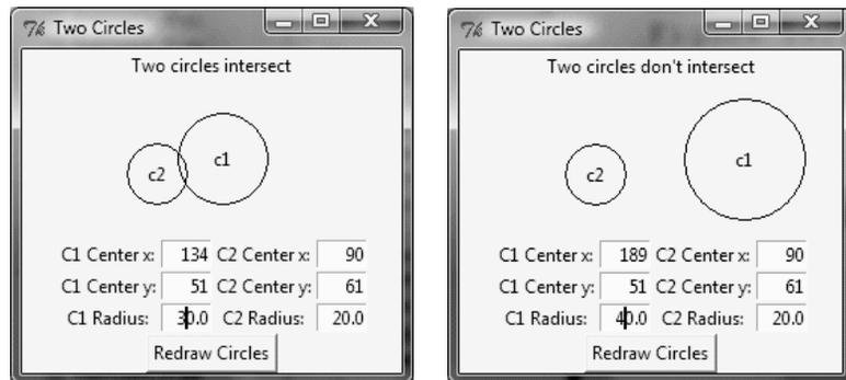
**FIGURE 12.20** Check whether two circles are overlapping.
