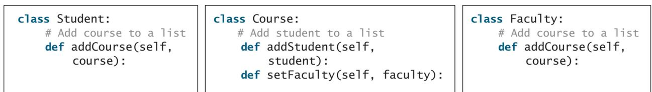
**FIGURE 12.6** The association relations are implemented using data fields and methods in classes.
