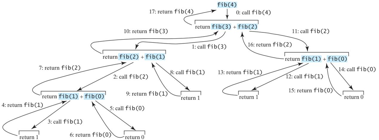
FIGURE 15.4 Invoking `fib(4)` spawns recursive calls to `fib`.
