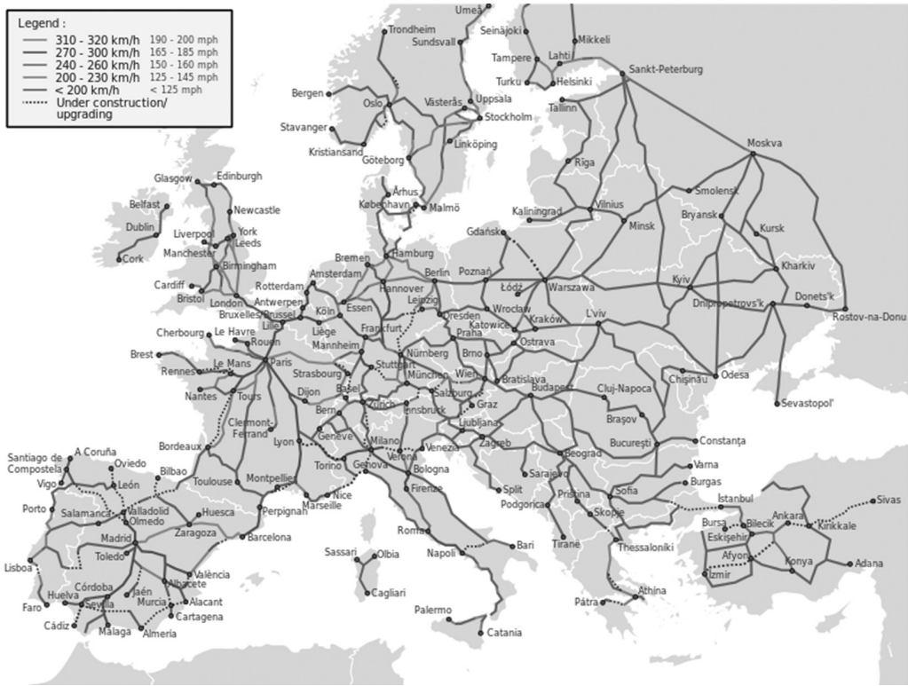
FIGURE 6.1 High-speed lines in Europe, 2014. (From Bernese Media and BIL, 2014, via Wikimedia Commons. Derived from High Speed Railroad Map Europe 2011.)
