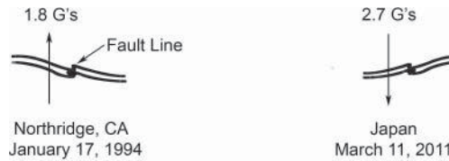
Figure 24 Earthquake plate action.
