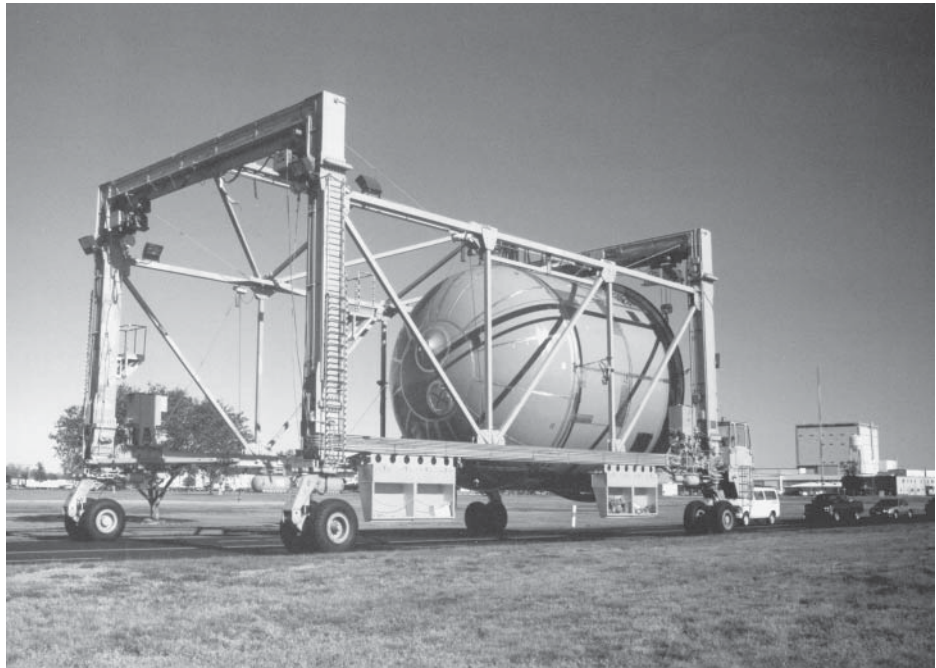
Figure 5 Fuel tanks and booster rockets such as those of the Space Shuttle are 2xxx alloys, originally 2219 and 2419, now Al–Li “Weldalite” alloy 2195. (Courtesy of the Aluminum Association.)
