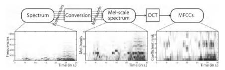
**Fig. 2.** Successive steps for the computation of MFCCs, illustrated with the analysis of an audio excerpt decomposed into frames.
