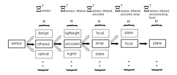
**Fig. 1.** Example for the relationships in  $\Xi_{\delta_1,...,\delta_{\mu}}^T$ : Uncooled infrared sensors can be build by using the focal plane array technology.
