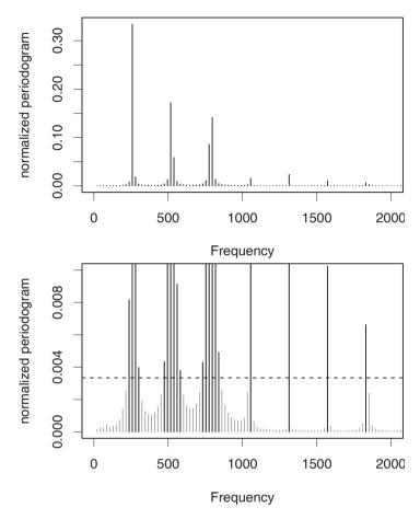
**Fig. 2.** Periodogram of note c4 played with an electric guitar. Original (upper part) and zoomed in with cut-off line (lower part)
