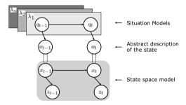
**Fig. 1.** Overview of the framework. At each time step t, the state  $x_t$  of the system is estimated from the observations  $z_t$ . A relational description  $o_t$  of the estimated state is generated and evaluated against the different situation models  $\lambda_1, \ldots, \lambda_n$ .
