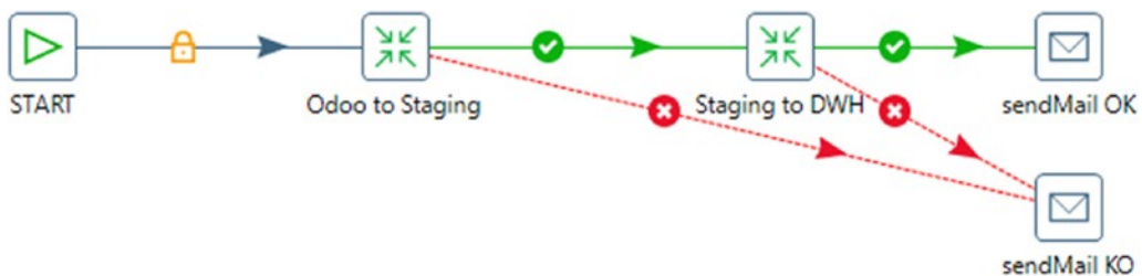
Figure 10-5. Linking both error outputs of the two transformations to the same sendMail step
