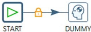
Figure 6-9. Linking steps. Once we clicked the “exit” button, we drag and drop the arrow to the next step
