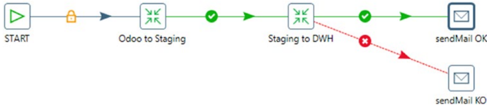
Figure 10-1. Connecting the steps in the canvas to create the job that will launch our both transformations
