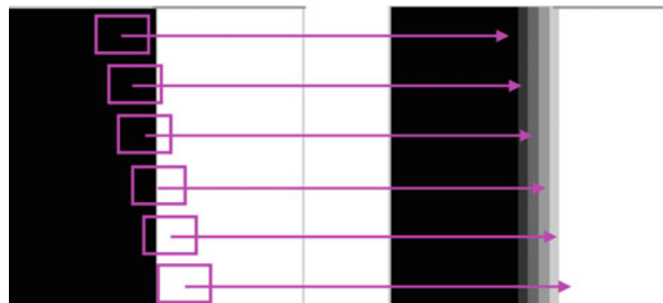
Fig. 4.12 An illustration of blurring after applying mean filter on the image edge (the mask size used is 5 \times 5 )
