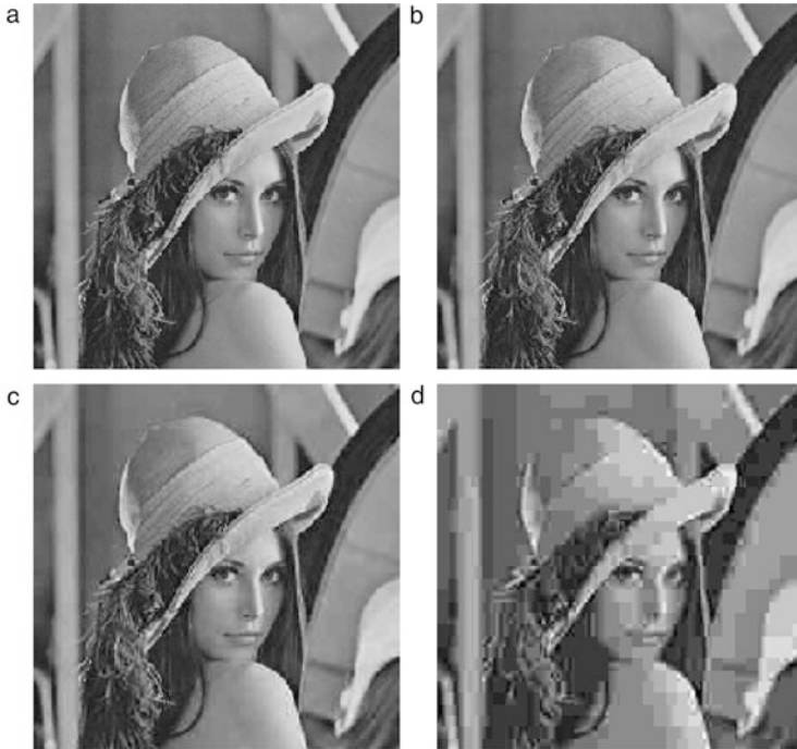
Fig. 4.25 (a) Original “Lena” image, (b) “Lena” image after applying JPEG compression with QF = 70\% , (c) “Lena” image after JPEG compression with QF = 25\% , (d) “Lena” image after JPEG compression with QF = 5\%
