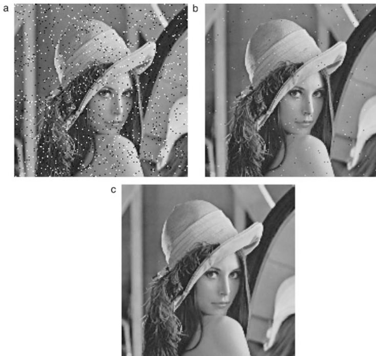
Fig. 4.16 (a) “Lena” affected by impulse noise with density 0.05, (b) denoised image (median filter of size 3 \times 3 is used), (c) denoised image ( 5 \times 5 median filter)
