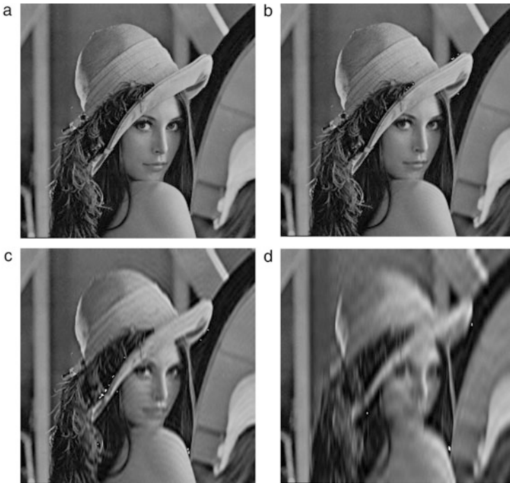
Fig. 4.19 (a) Original image “Lena” (b) image based on the first 128 \times 128 DCT coefficients, (c) image based on the first 64 \times 64 DCT coefficients, (d) image based on the first 25 \times 25 DCT coefficients
